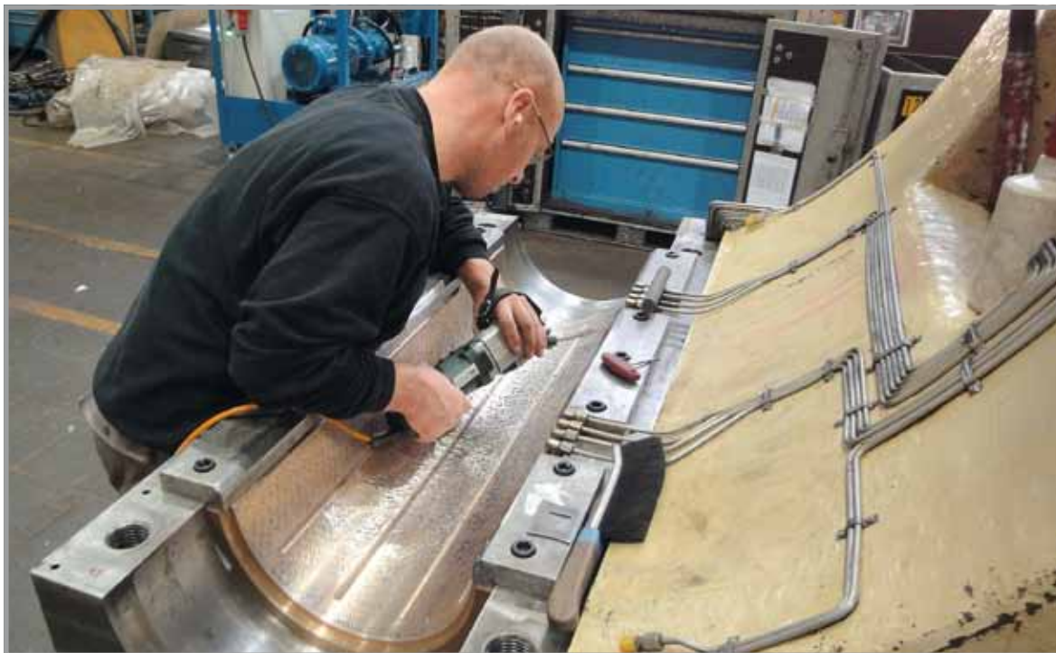
The heart of the machine – the pressram – is scraped in order to guarantee the high demands placed on the machine parts.
