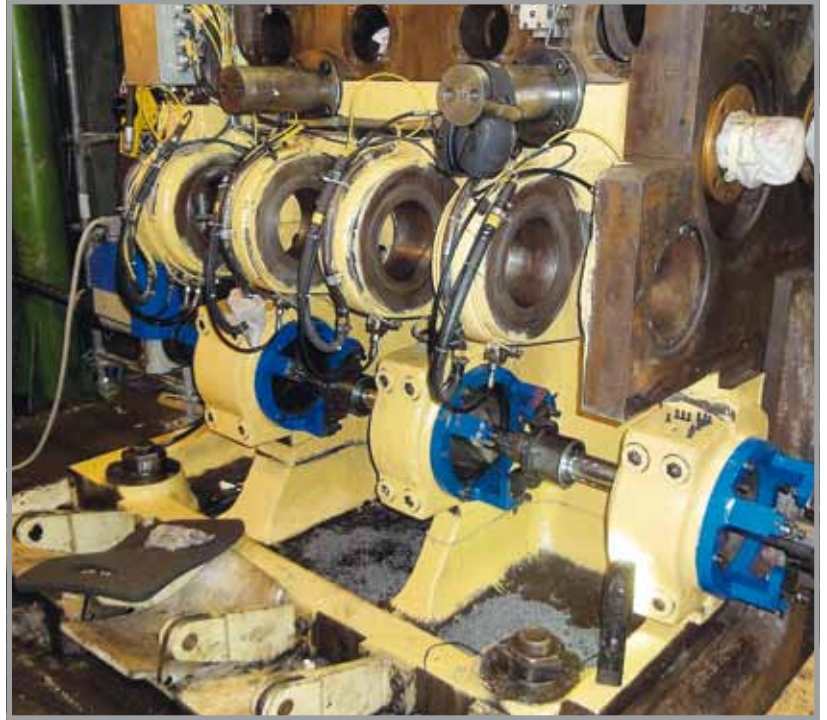
The ejector shaft area with multiple upper and lower bearing points is machined in one setting.
