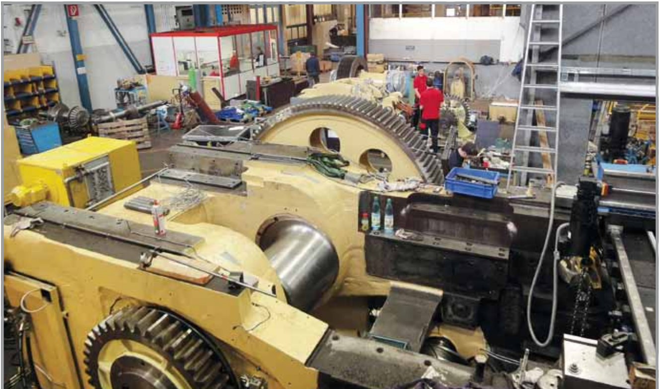
The ejector shaft area with multiple upper and lower bearing points is machined in one setting.
