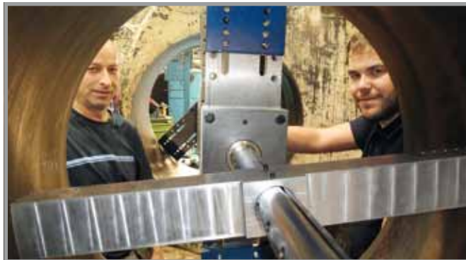
First-time re-machining of the crankshaft bore.
