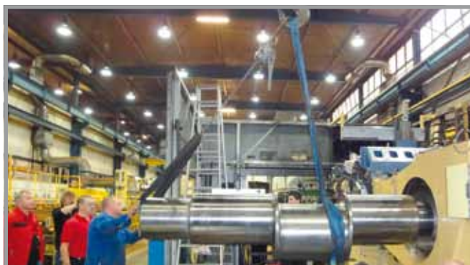
The crankshaft can then be refitted with a new bearing.
