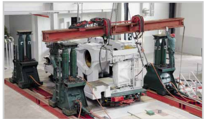
Extremely concentrated work is needed for the final few meters, in order for the machine to be placed in the correct position. The alignment of the leveling and damping elements by the Hatebur engineers (photos in order starting at top left) is also extremely important.
