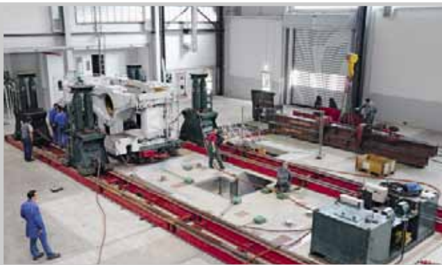
Extremely concentrated work is needed for the final few meters, in order for the machine to be placed in the correct position. The alignment of the leveling and damping elements by the Hatebur engineers (photos in order starting at top left) is also extremely important.
