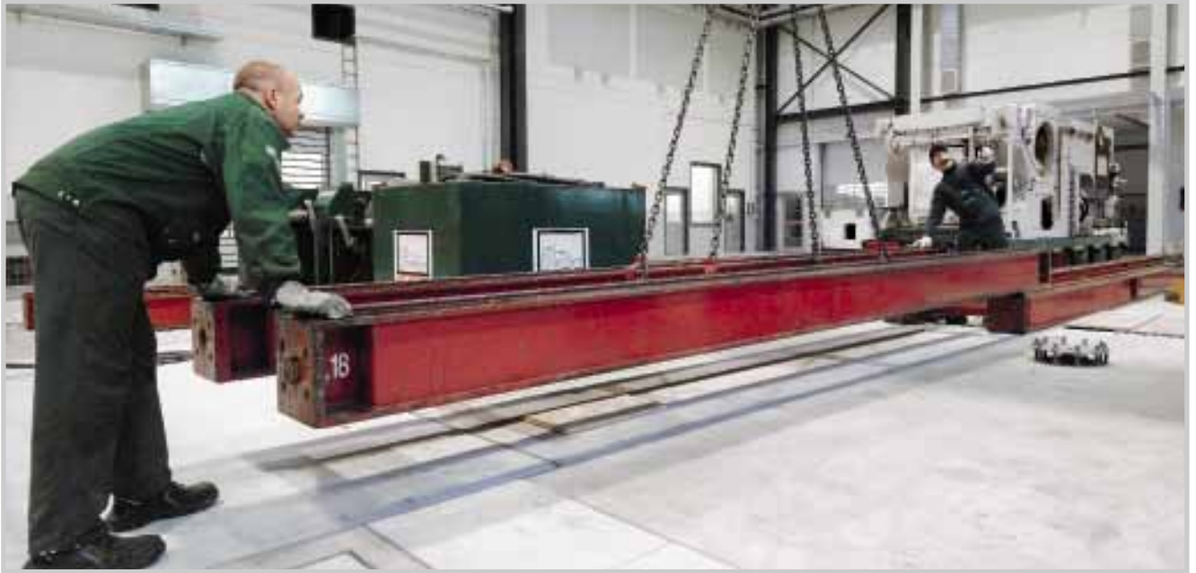
The machine is pulled into its final position on the precisely aligned rail system.
