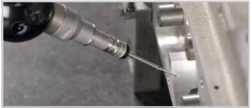
The tolerance of components is tested on random samples on calibrated measuring tables.
