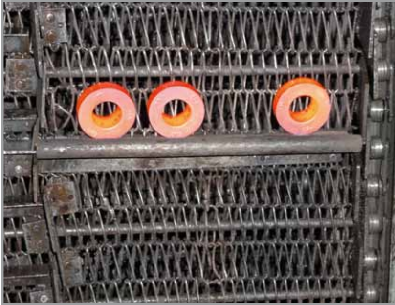
The new parts are still hot during transport to the discharge.
