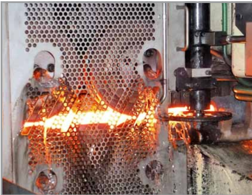
The servo-driven infeed rolls bring the heated bar into the machine.
