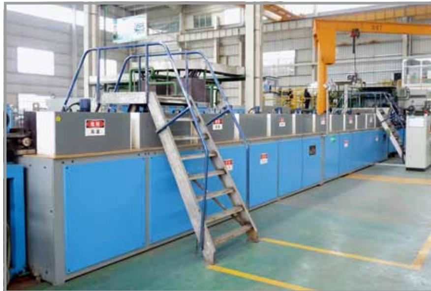
The bar heater of the AMP 70.
