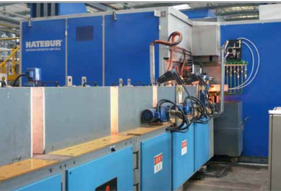
The bar heater of the AMP 50.
