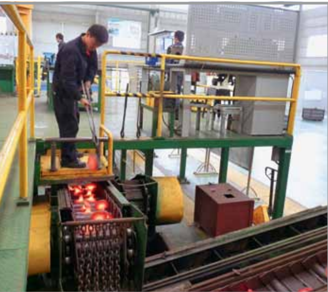
The forging (hub blanks) on the inspection conveyor.
