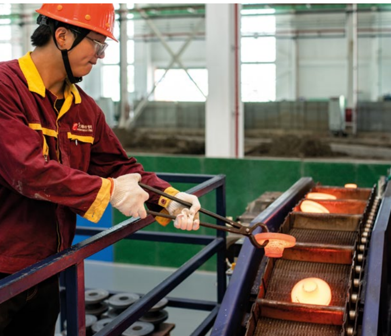
➤ Currently, the company uses the HOTmatic HM 75 XL to produce flanges. In the future, it will manufacture precision parts for the automotive and electric mobility sector.
