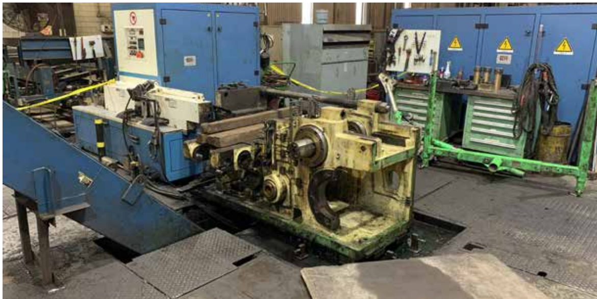
➤ From old to new – step 1: The old Hatebur AMP 20 stripped to its frame and ready for removal.
