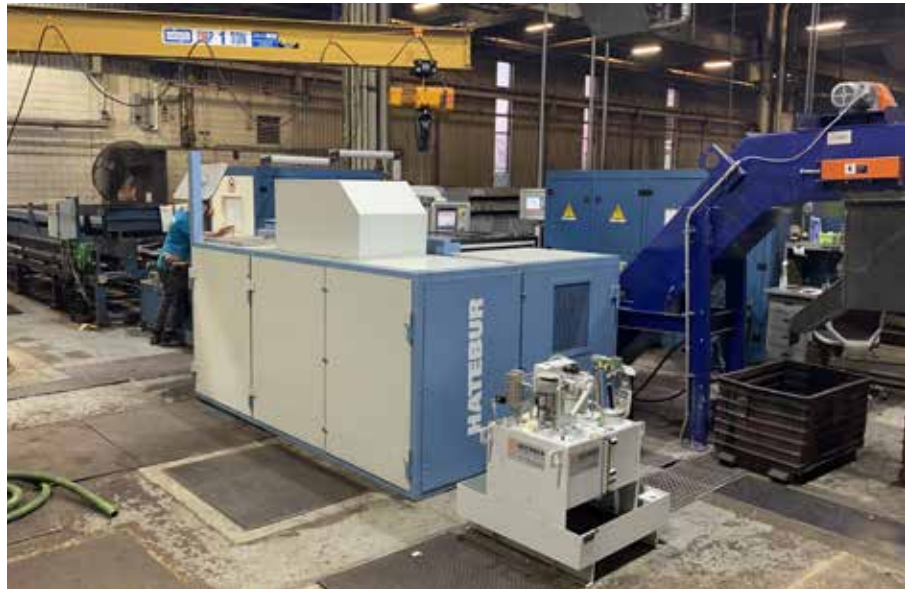
From old to new – step 3: the new Hatebur HOTmatic AMP 20 N, including the sound enclosure.
