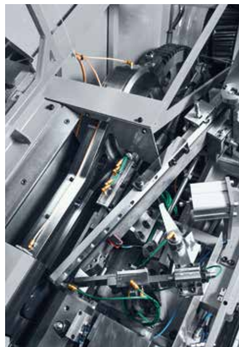
➤ Heading Unit Proven Carlo Salvi quality: The five-station header shines with flexibility, efficiency, precision and user friendliness.
