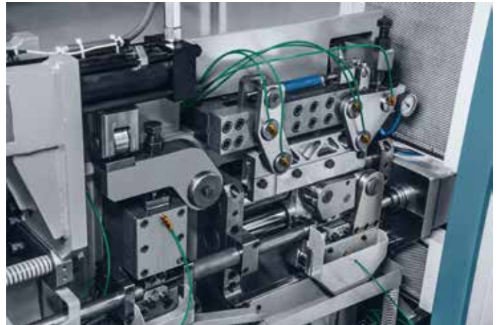
➤ Linear Wire Feed: The linear wire feed ensures the highest level of precision for the cut-off blank.
