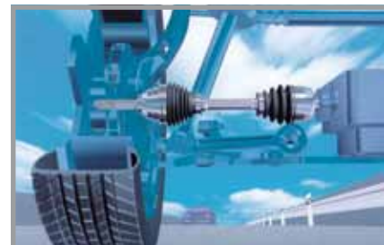
Basic principle of a constant velocity drive shaft in a passenger vehicle.
