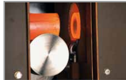
The induction heater used on the HM 75 has a throughput of 15 tons/hour.
