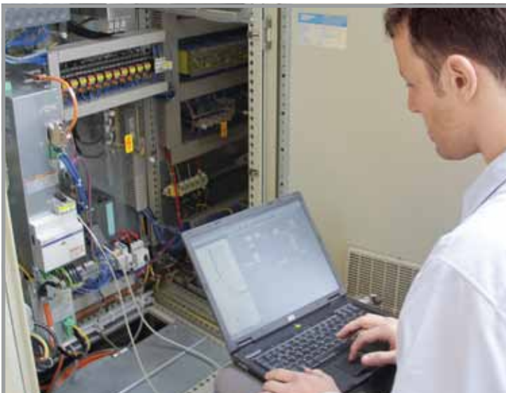
Oliver Maritz programs the SPS interface of a servocontroller on a test setup.
