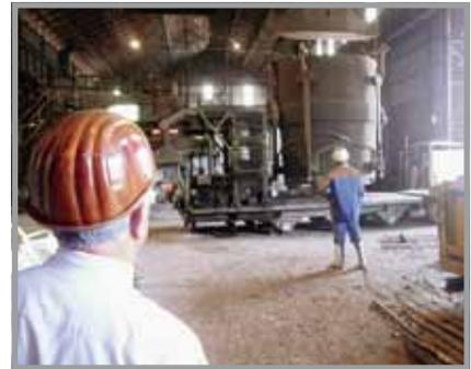
*Exactly the same process is used with the second casting ladle, which is also moved into position next to the 35-ton furnace, and filled.*
