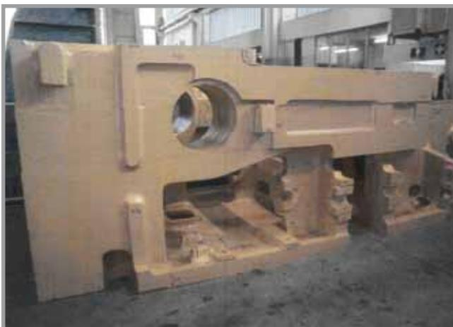
*In mechanical processing, the feeder system is separated and the body is sand-blasted before being rough-machined and primed. Only then is the body ready for normal further processing to become the next Hatebur machine.*
