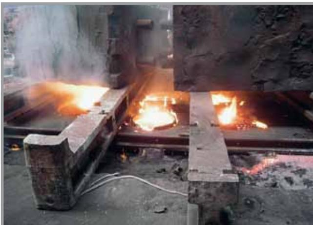
*The cast now has to rest for two weeks in the earth until it has cooled down.*
