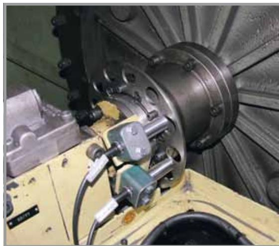
*The standstill monitor and locking systems from Garrison and Schmersal are necessary and an essential component for complying with the statutory regulations of the machine guidelines.*
