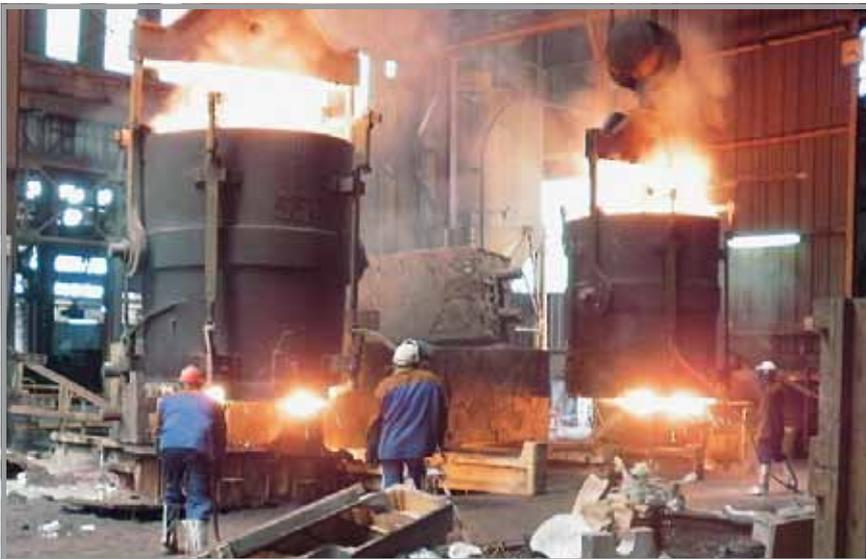
*The teams for the two casting ladles come to their final agreement on how to proceed, then it's down to business. The two casting ladles must be positioned precisely over the openings of the mold, which requires precision work!*
