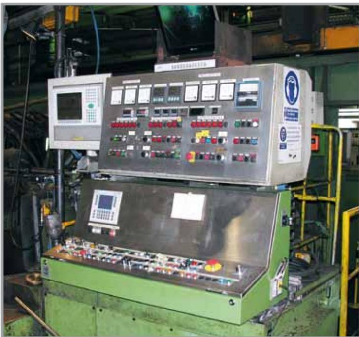
*The newly positioned and installed control for the machine, the ESA600, press load monitor and the heating unit.*
