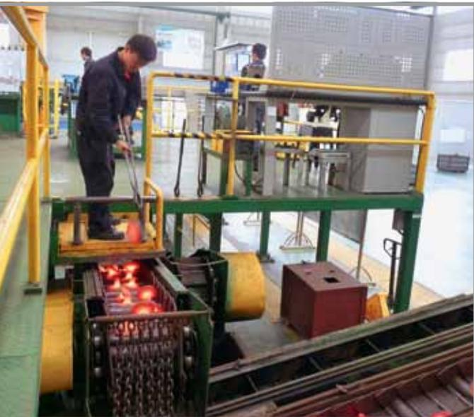
*The forging (hub blanks) on the inspection conveyor.*
