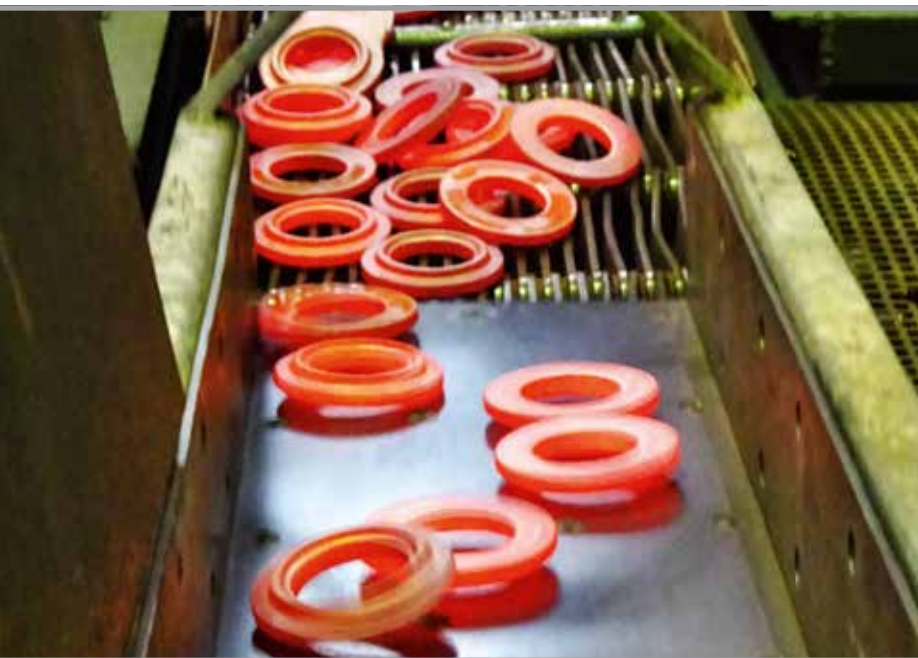
A conveyor belt several meters long transports the hot parts.
