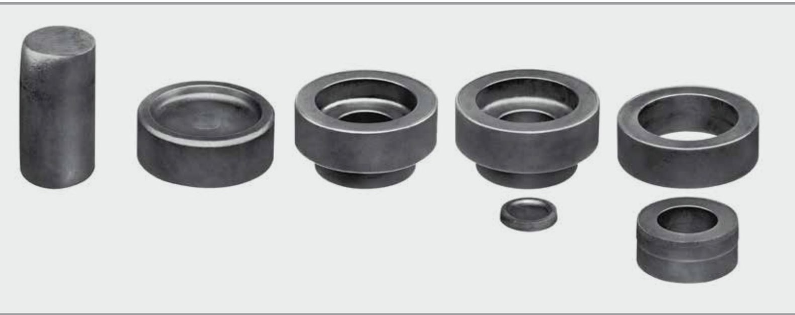
New sequence of operations for the production of combination rings on the AMP 50-9.
