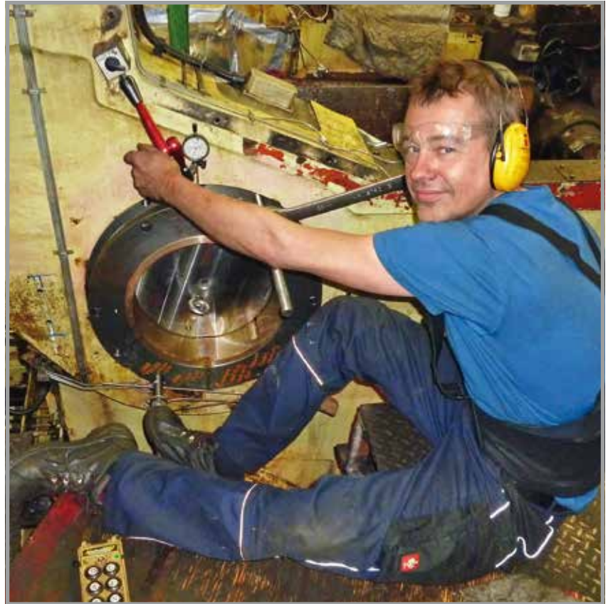
Hatebur service engineer Matthias Aebi measures the fit between the crankshaft bore and the crankshaft sleeve on 4th station side.
