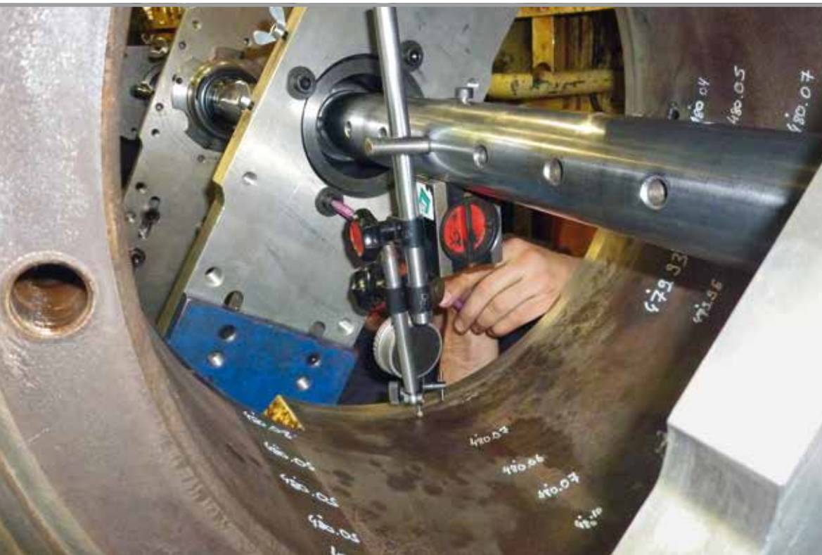
The crank house bores were re-bored for the first time since the AMP 40 is in production (1989).
