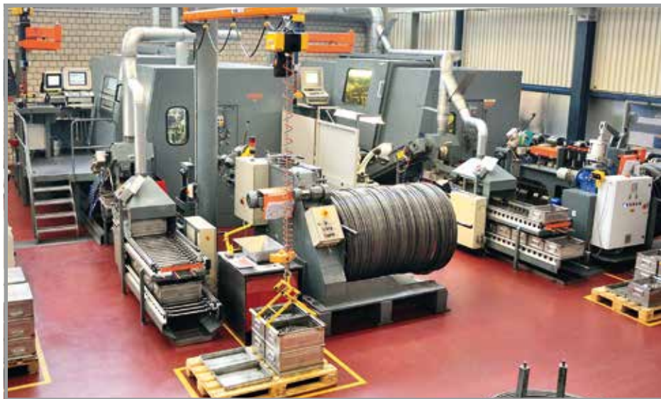
View of a Hatebur Coldmatic in an SFS production facility.
