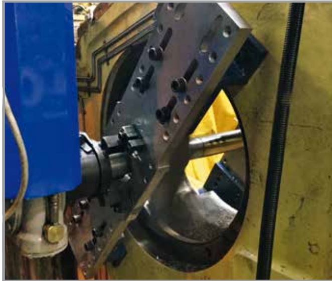
Machine device for the machining of the 1st station crankshaft bore.
